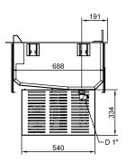
D = Drain EI = Electrical inlet (power)
